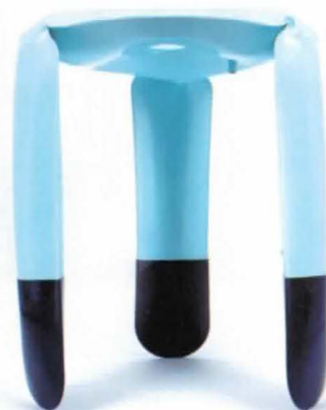
The Stool , the idea was to produce stable and convenient furniture out of thin metal sheets using the potential of CNC machines and hydro formed metal surfaces. The hydro-formed process applies liquids with high pressure to the water-tight welded inner space. This pressure and the thickness of the metal sheets define the 3D appearance and stability of the chair. Design: Oskar Zieta www.zieta.pl
